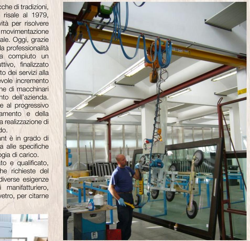
**PANNELLI****PANELS / PANNEAUX**
